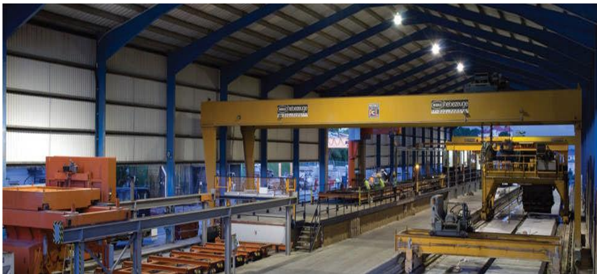
Figure 3.10: Pre-fabrication of Deck Panels in Plants (Bostwana, South Africa)
