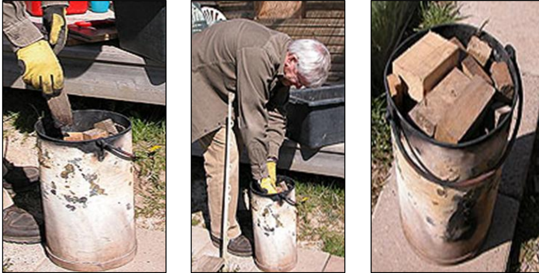
Fig 3.3: Fill the smaller vessel with biomass
