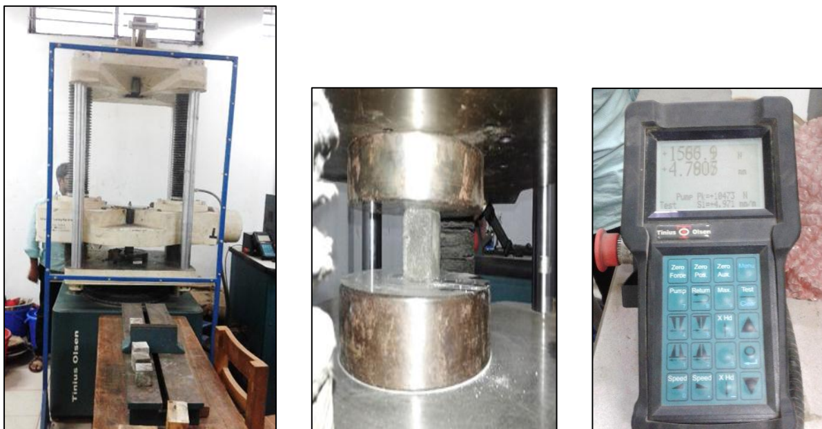
Fig 3.39: UTM machine, load applying and recording
