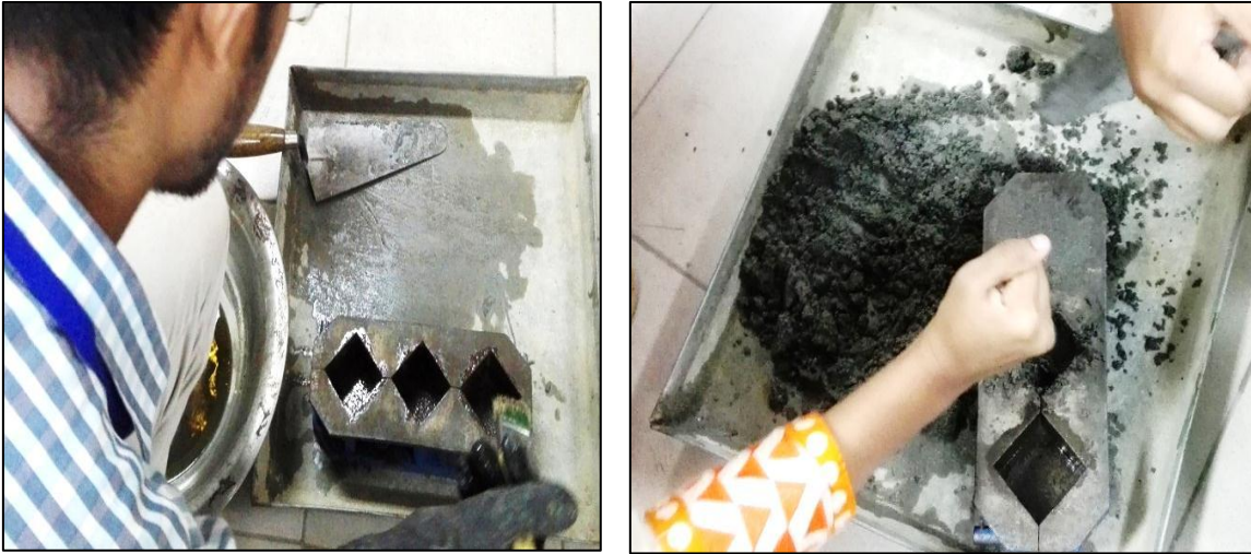
Fig 3.33: Lubricate mold and place & compact the sample
