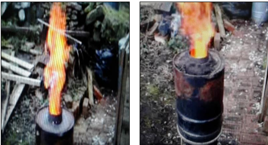
Fig 3.15: Smoke gone and large flame appear
