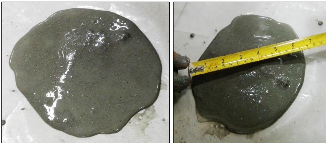
Fig 3.51: Measure the sample diameter after spreading
