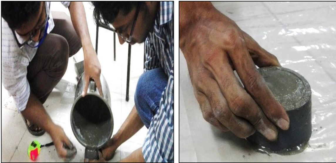
Fig 3.50: First molding & then demolding
