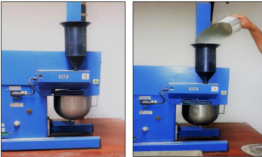
Fig 3.32: Thoroughly mix the materials by automatic mixing machine
