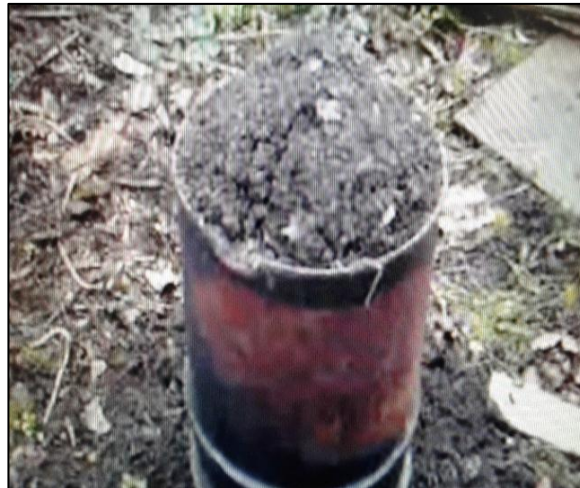
Fig 3.16: Top of the barrel filled with soil to prevent spontaneous combustion
