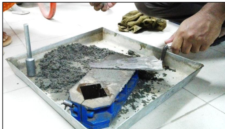
Fig 3.35: Level the mixture with trowel
