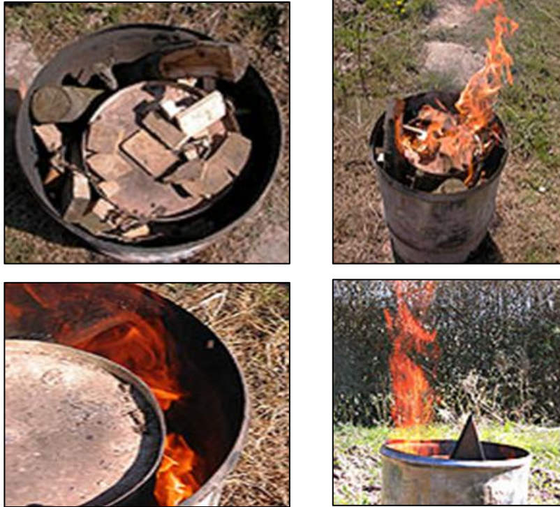
Fig 3.6: Burn the wood placed in the outer barrel
