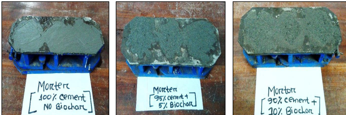
Fig 3.36: Casting & molding is complete
