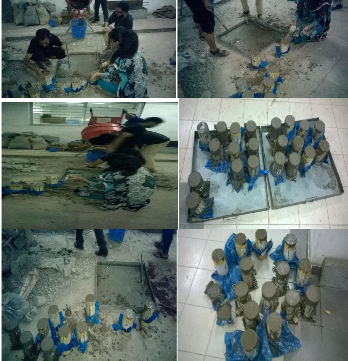
Fig 5. filled cylindrical mold with prepared concrete .
