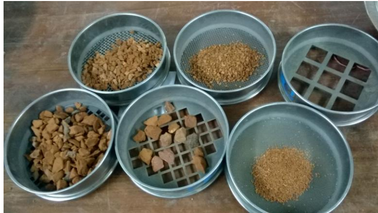
Fig 5.4: After sieve analysis of Brick chips
