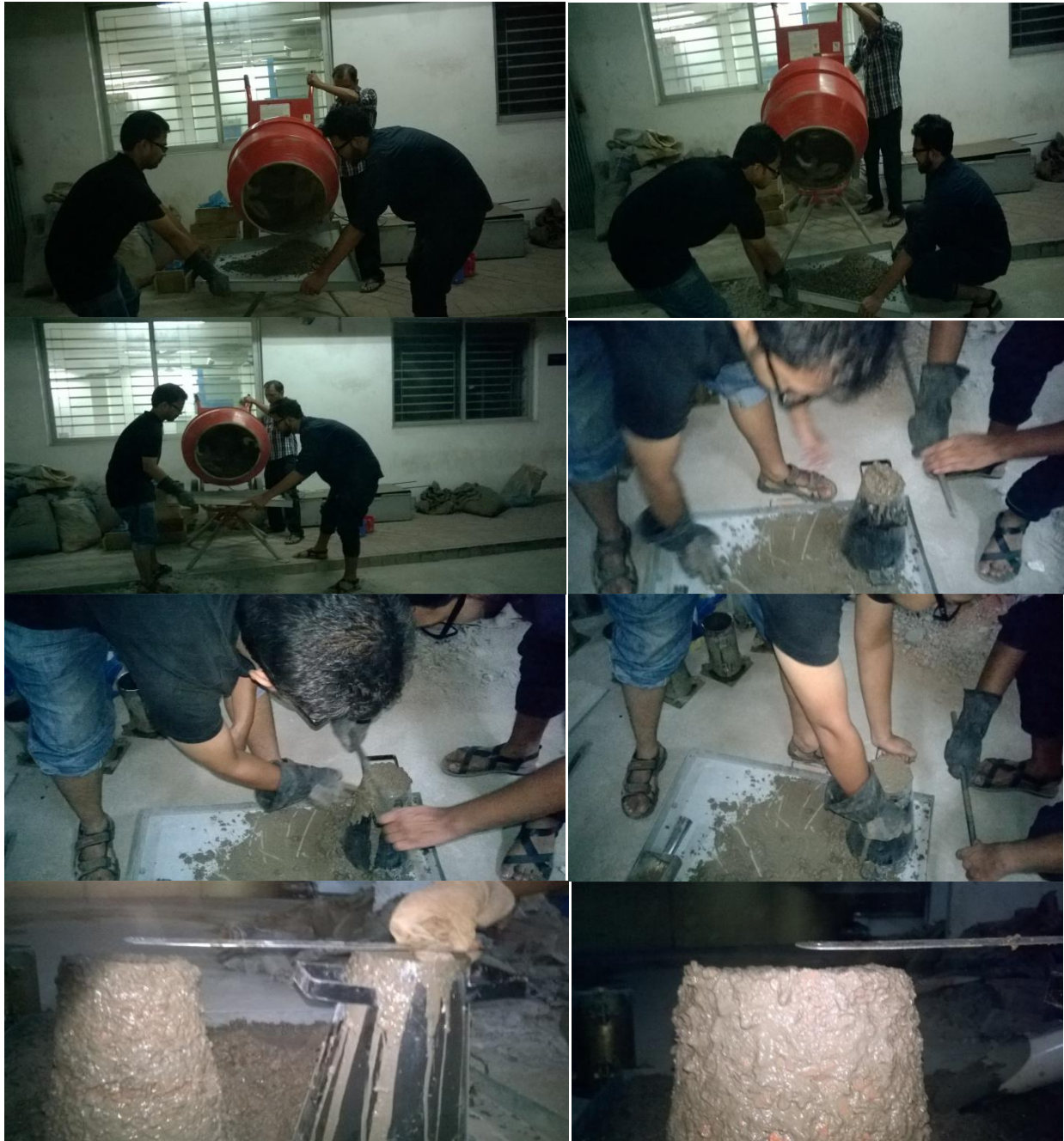
Fig 4. Prepared concrete, slump test.
