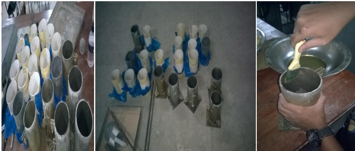
Fig 3. Preparation of mold
