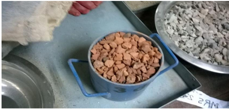
Fig 5.1: finding of void% for brick chips
