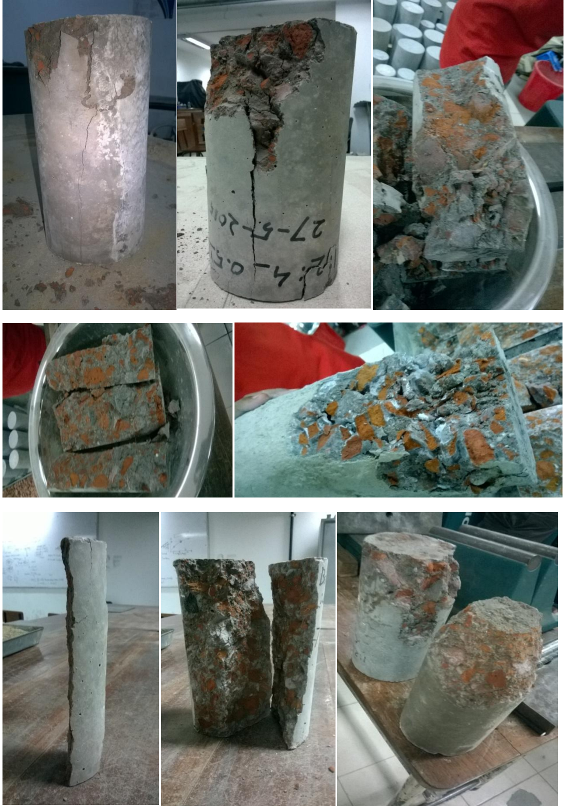
Fig 8. Failure surface of concrete.
