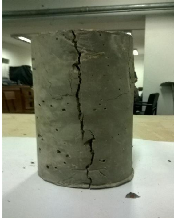
Fig 5.29: breaking of cylinder (4inchX8inch)
