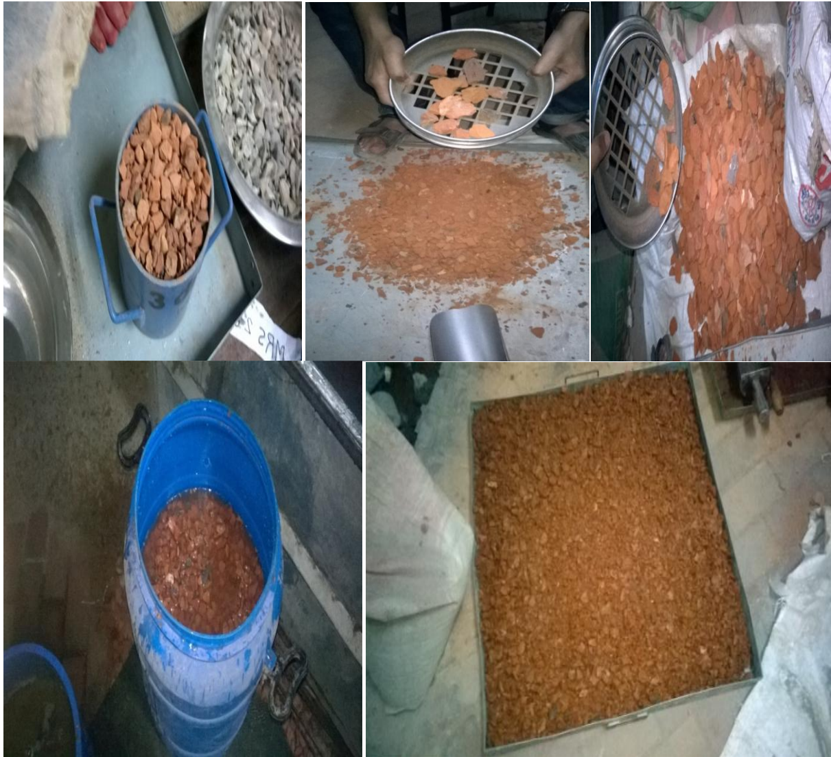
Fig 1: preparation of brick chips
