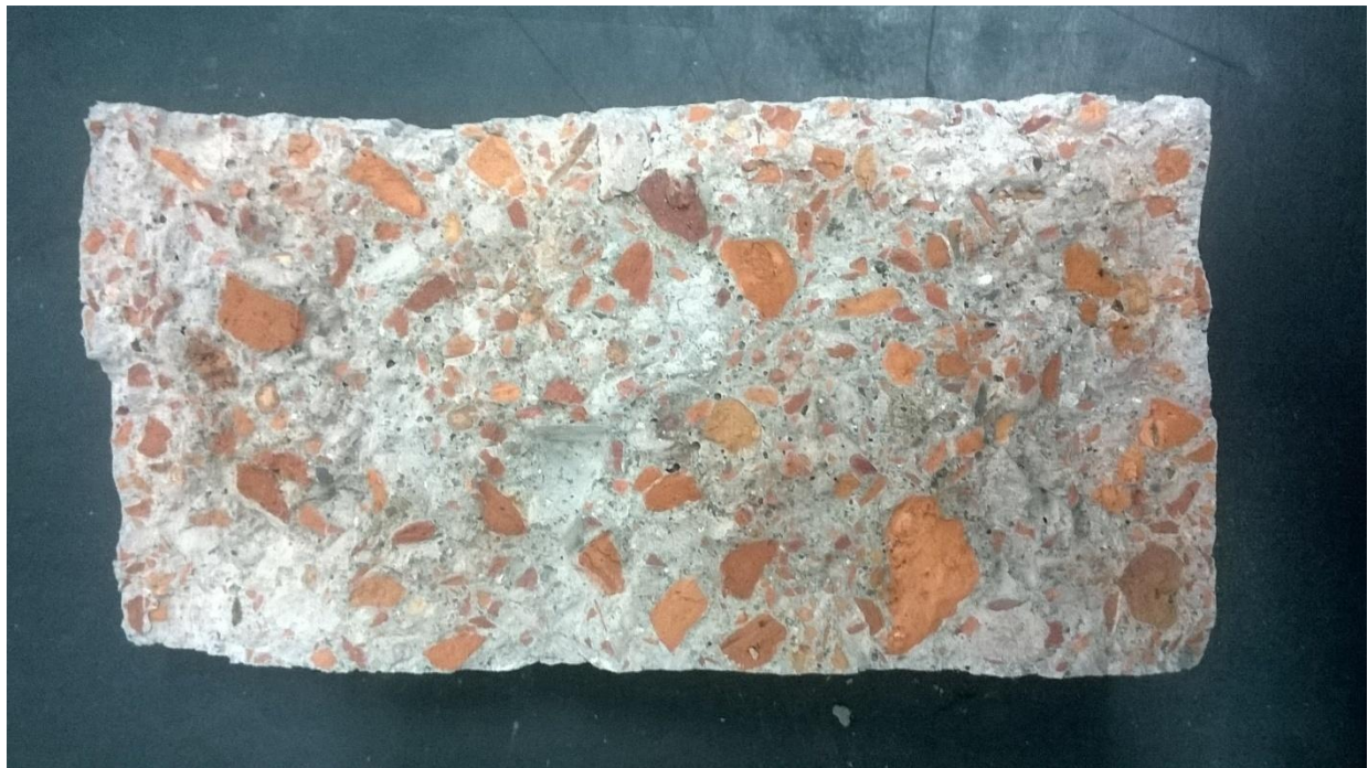
Fig 5.30: After breaking of Cylinder
