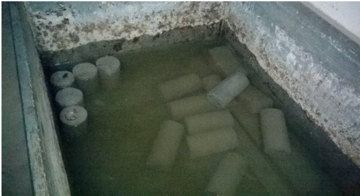
Fig 6. Concrete separated from mold & submerged into water
