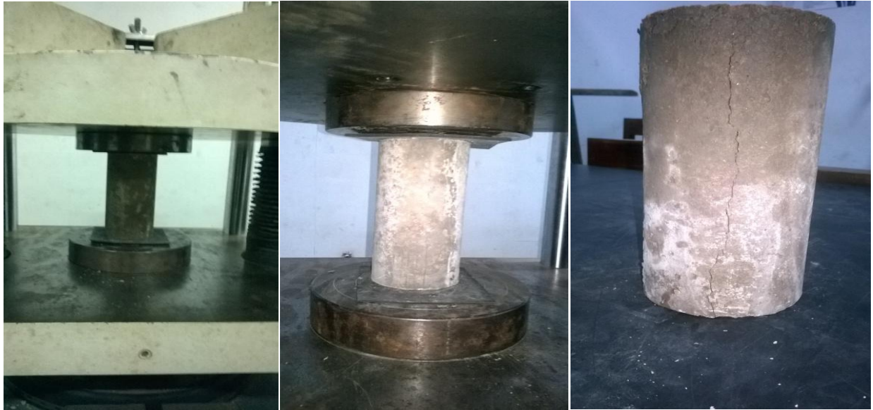
Fig 7. Compressive strength test
