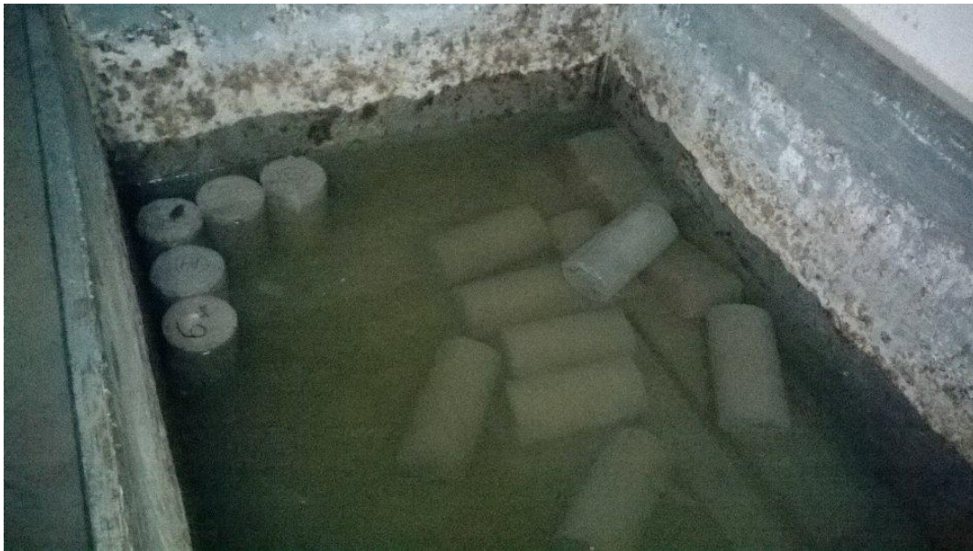
Figure 4.1: Mold are submerged into water tank
