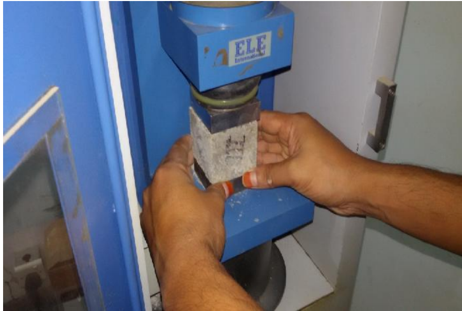
Figure A8 :- Placing sample into crushing machine
