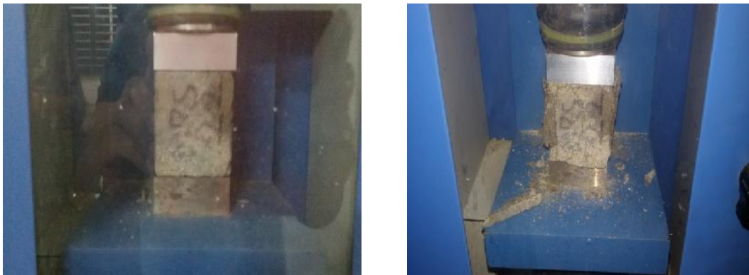
Figure A9 :- Sample Crushing
