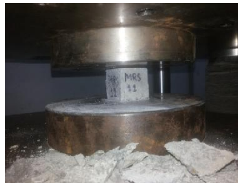
Figure A7 :- Sample crushing by UTM machine
