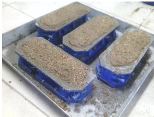
Figure A5 :- After casting, wet sand and wet cloth has been placed above sample to prevent moisture loss.
