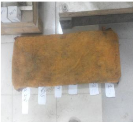
Figure A5 :- After casting, wet sand and wet cloth has been placed above sample to prevent moisture loss.
