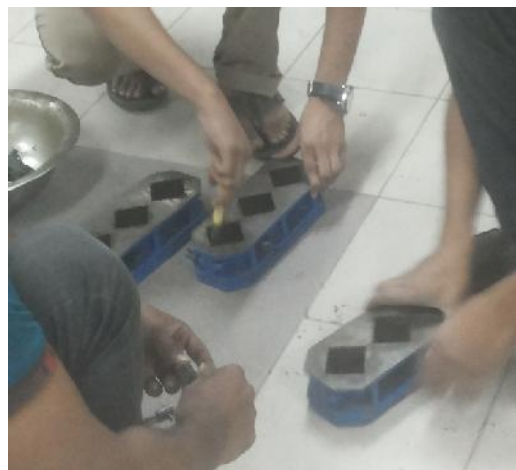
Figure A2 :- Mold Preparation for Casting
